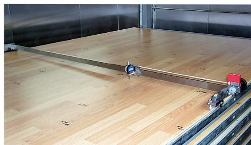
Testing rack of IHD with measuring bridge (test area 3 m x 2 m)
