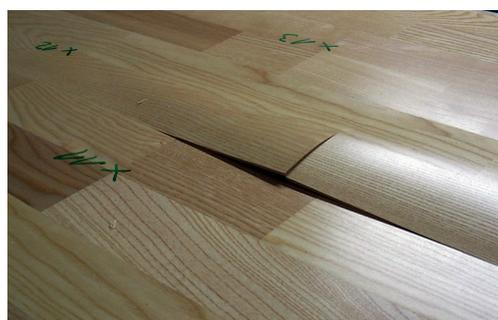
Delamination between layers of a flooring construction
