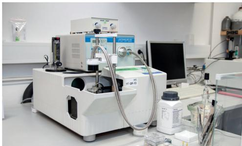
Determination of the glass transition temperature
