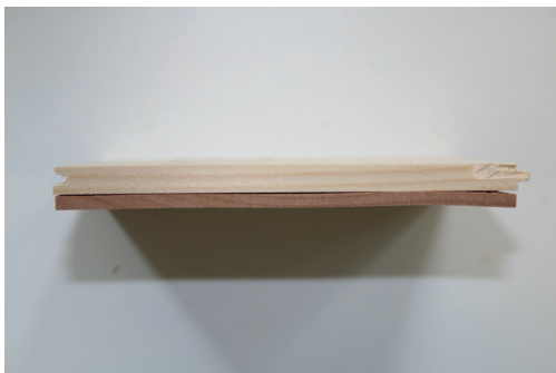
Delaminated specimen, after storage in drying oven
