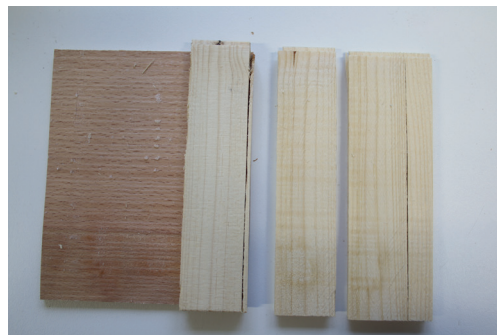
Detected glue-failure, after alternating conditioning
