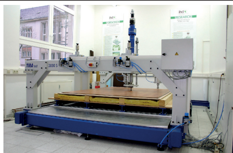
System testing machine – testing of a complete ceiling structure
