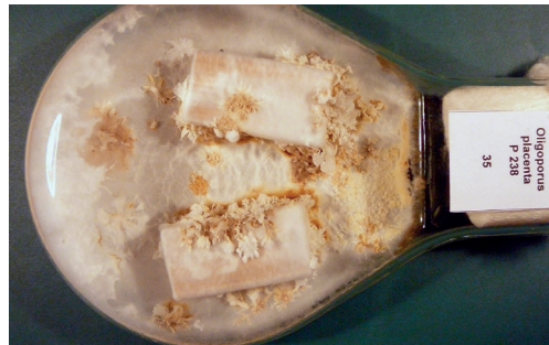
Fungus test of Thermally Modified Timber (TMT)
