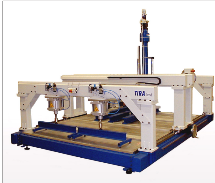
Test of structural flooring on joists
