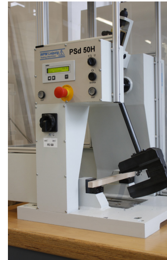
Testing of impact bending strength
