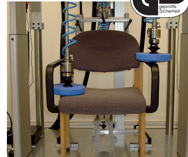
Arm rest static load test
