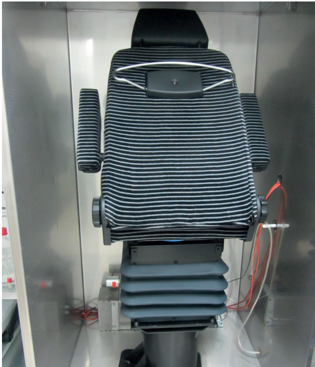
Determination of VOC and formaldehyde emission from a driver's seat
