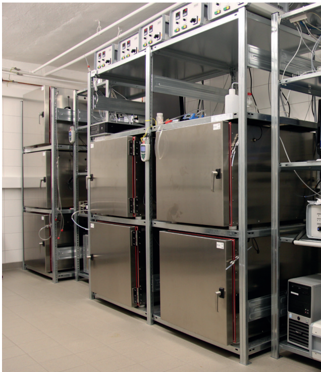
Small test chambers for determining formaldehyde emissions acc. to ASTM D 6007 and VOC emissions e.g. acc. to EN 16516
